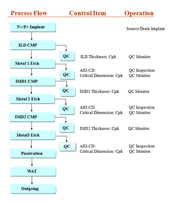
Figure 3.1 Generic SRAM Wafer Process & Control
