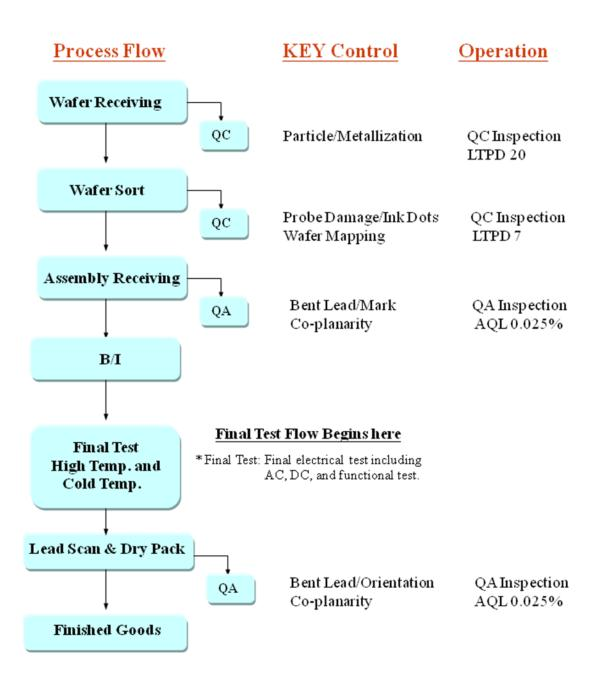
Figure 3-4 Commercial DRAM Test Flow & Control
