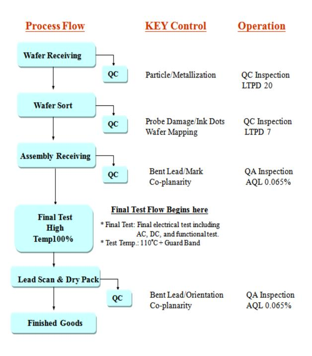
Figure 3-5 Commercial Flash Test Flow & Control
