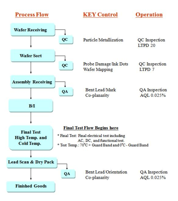
Figure 3-3 Commercial SRAM Test Flow & Control
