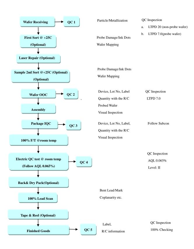
Figure 3-6 Commercial Analog Test Flow & Control
